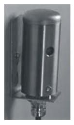
The DURLUX-T 4-20mA measure the ambient illuminance -lux- and converts it to a current loop signal.
