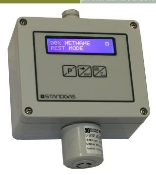
Standalone programmable detector designed for the detection of explosive gases using catalytic technology (pellistor), with a detection range of 0 to 100% L.E.L. and resistant to silicone vapours.
