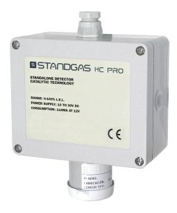
**Stand–alone detector** for industrial use designed for the detection of explosive gases using catalytic technology (pellistor), for a detection range of 0 to 100% L.E.L and resistant to silicone vapours.
