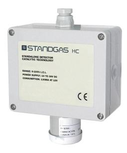
**Stand–alone detector** designed for the detection of explosive gases using catalytic technology (pellistor), for a detection range of 0 to 100% L.E.L and resistant to silicone vapours. It is also available in a special version with three programmable relay outputs.
