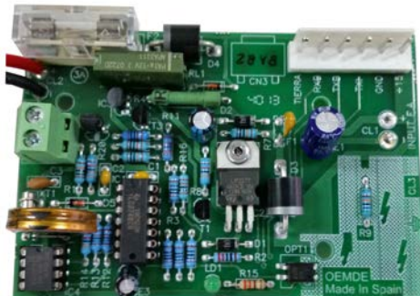
Power Supply Control Module.
