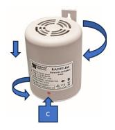
**8.** To close it, position the body on the support with the LED (C) and specs label facing the front. Turn slightly to the left until it slots into the base. Finally turn clockwise until it reaches a stop.
