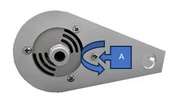
**1.** Using a 3mm Allen key, loosen the locking screw **(A)** which allows the detector to be opened by turning it anticlockwise.
