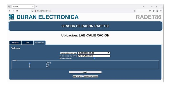
Parameters: Set time and date, Assign detector location, change operating mode, autonomous or connected to a **DURGAS** control panel, select different relay states AUTO-ON-OFF, factory reset and firmware update. When you change any of the options confirm with Apply, to update the equipment's firmware consult page 11 and follow the instructions.
