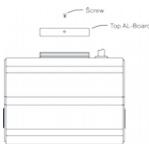
2. Secure aluminium mounting piece to ceiling or wall with screws.
