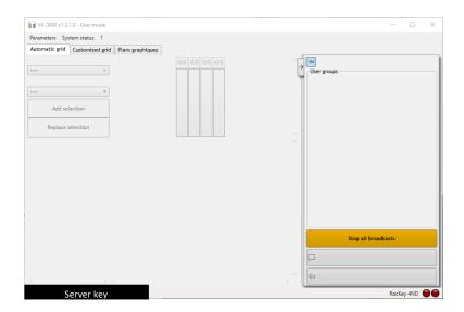
The Audio Management Software is to be configured by the installer before it can be used by the enduser. The software has an administrator mode for configurating the settings and the user interface and a user mode for operating the system. The user mode can be utilised either with a grid ("automatic or customized grid") or a customised building map ("plans graphique", in the following "map view") which is more convenient for external or beginner users.
