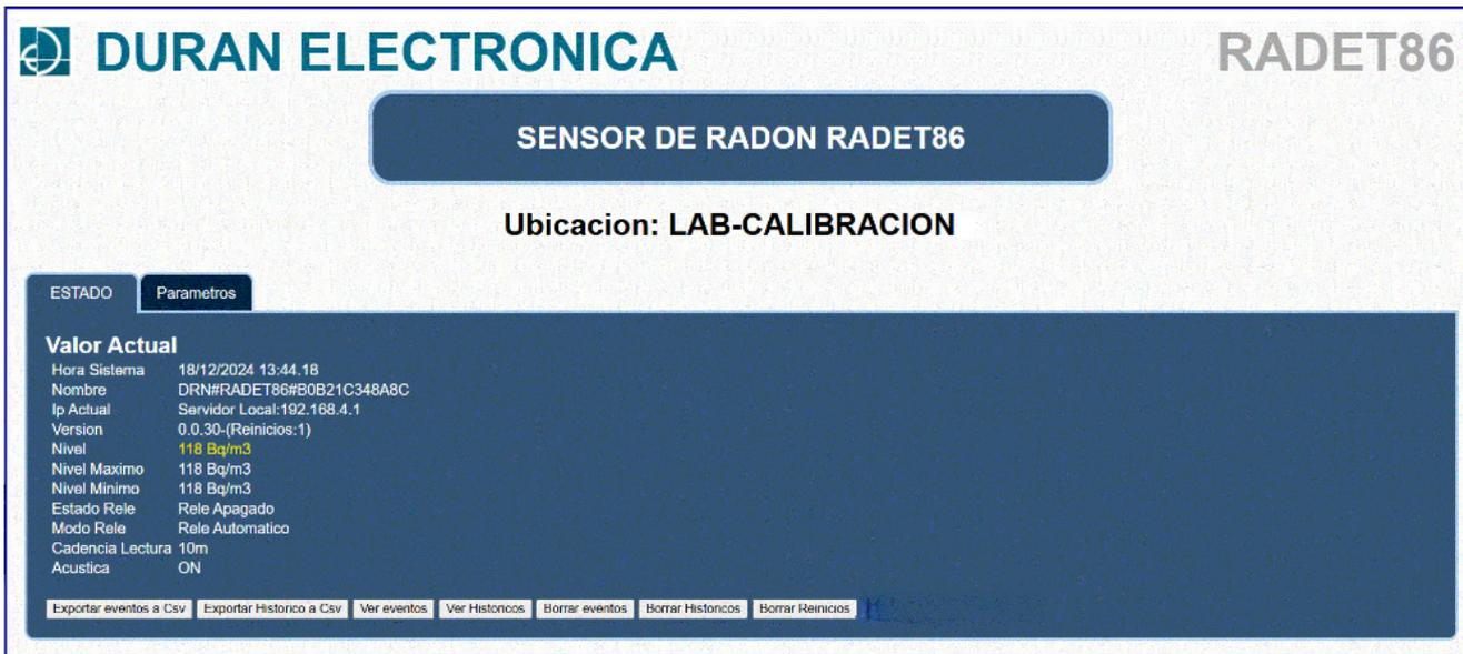
The screenshot shows the web interface for the RADET86 detector. At the top, it displays the DURAN ELECTRONICA logo and the model name RADET86. Below this, a dark blue button reads 'SENSOR DE RADON RADET86'. Underneath, the location is specified as 'Ubicacion: LAB-CALIBRACION'. The interface is divided into two tabs: 'ESTADO' (selected) and 'Parámetros'. Under the 'ESTADO' tab, there is a section titled 'Valor Actual' with the following data:
